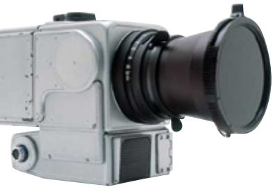
ZEISS Distagon 4/40 on the Hasselblad 500 EL moon camera
