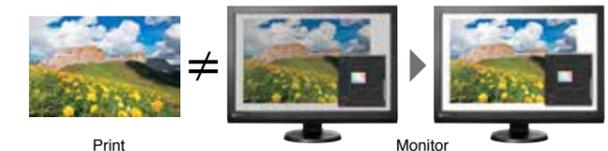
Adjust the **2 White Point**. Move the pointer to the left or right until it approximates the appearance of the print. If the screen output seems blue, move the pointer away from the blue spectrum and toward the red end of the spectrum to remove excess blue.
