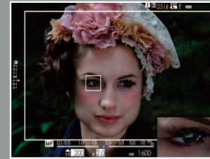
Digital Split Image can be selected in both monochrome and colour options
